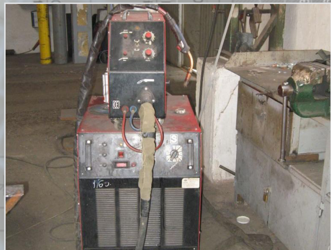
Welding machines (17 pieces) 400-600 A (for number 111, 133, 135 welding procedures)
