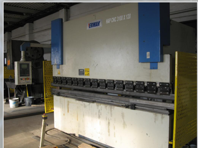
CNC controlled bending machines Length: 3.000 mm, thickness: 12 mm
