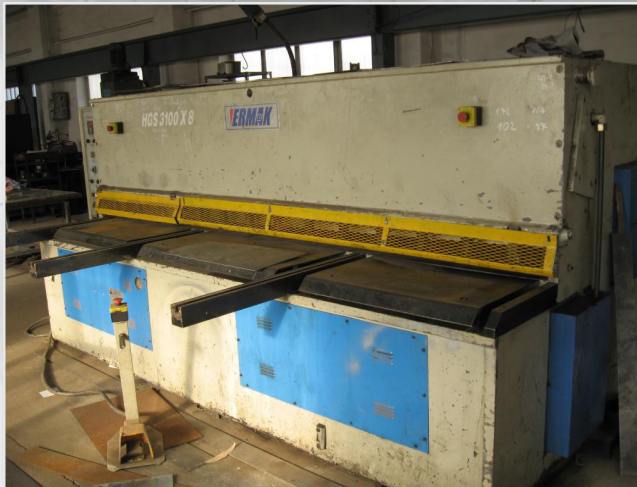
CNC controlled cutting machines (2 pieces) Length: 3.000 mm, plate thickness: 8 mm, 12 mm
