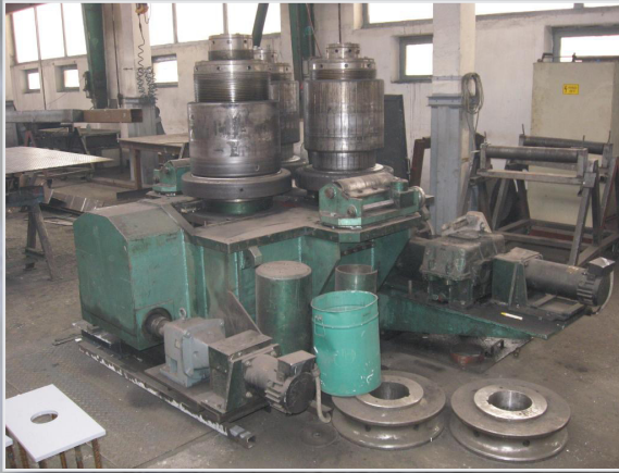
Special designed bending machine for H, I profiles up to 200 mm, minimal radius 6.000 mm
