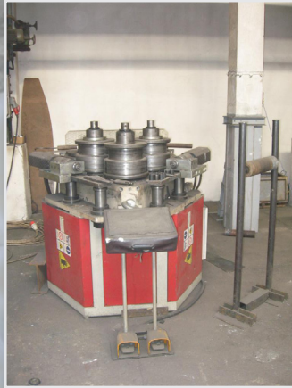
Hydraulic bending machines specially for flat steels, square tubes, round steels up to 100mm, minimal radius 500mm
