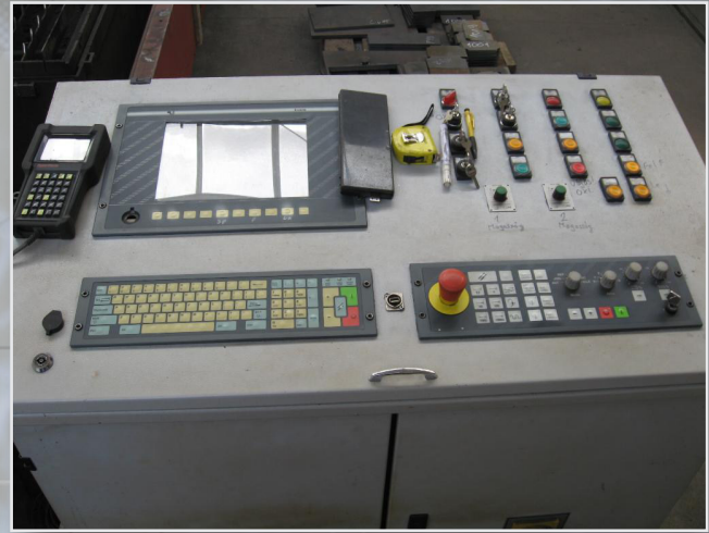
High precision steel sheet cutting machine Max dimensions: 2.000 x 6.000 mm , max sheet thickness 100 mm in case of burning and 20mm in case of plasma head.
