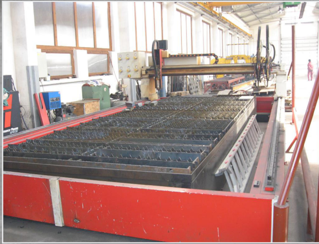
High precision steel sheet cutting machine Max dimensions: 2.000 x 6.000 mm , max sheet thickness 100 mm in case of burning and 20mm in case of plasma head.
