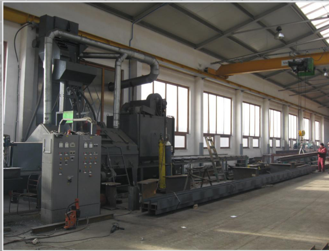
Sand blasting machine for surface treatment: up to 1.000 x 450 mm cross-section dimensioned structures or profiles
