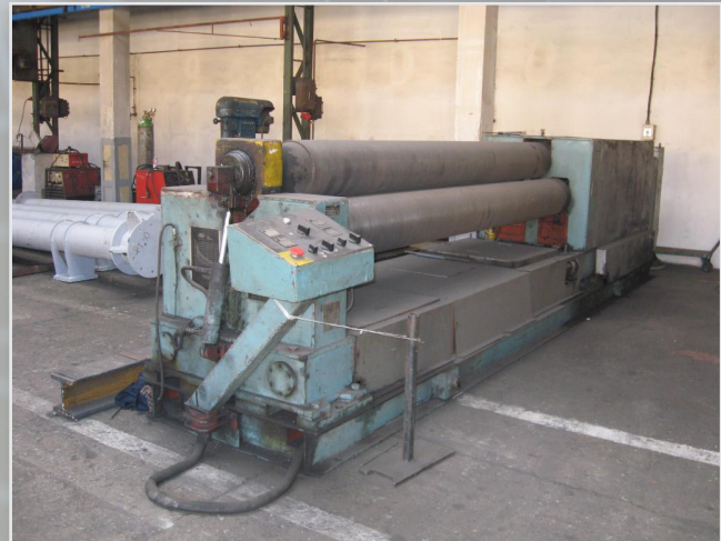
Sheet rolling machines (2 pieces) Length: 3.000 mm, thickness (in max length): 10 mm
