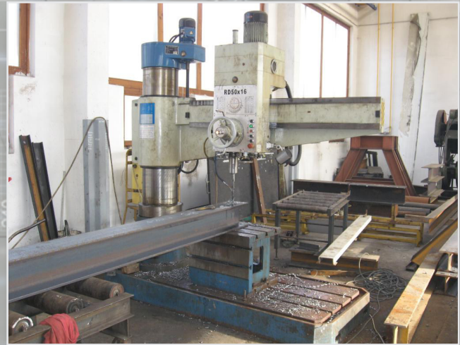
Radius drilling machine High precision boring
