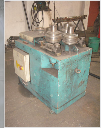
Hydraulic bending machines specially for flat steels, square tubes, round steels up to 100mm, minimal radius 500mm
