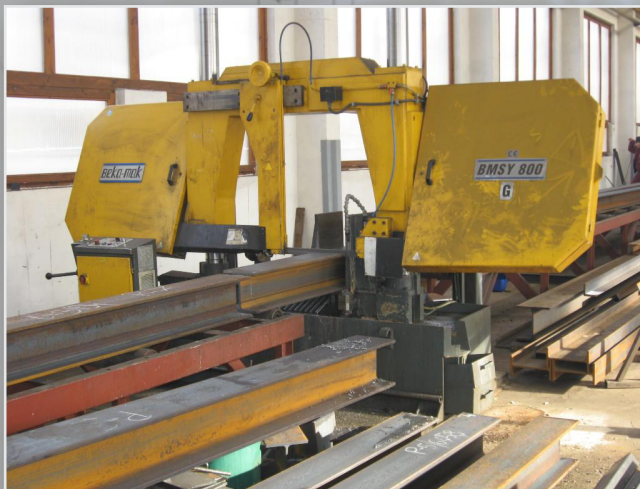
Profile cutting machines for profiles up to 800 mm (7 pieces)
